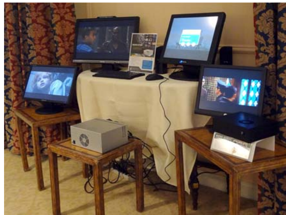
Figure Above: Live Demo Unit presented at the gaming conference in Las Vegas, 2011. BI355-67QM Industrial Computer (MX67QM mini-ITX motherboard inside) with Intel® Core i7 processor supports four monitors playing different HD content.
