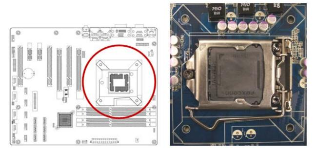
2. Unlatch the "CPU Socket Lever" by pressing the lever down and move it away from the main structure of the socket.
