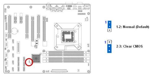
1. You can clear CMOS by shorting pin 2-3 for at least 30 seconds (while the system is OFF), then place the jumper back to pin 1-2 for normal operation.
