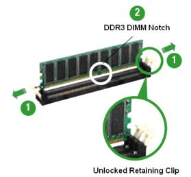
3. Firmly insert the DIMM into the socket until the retaining clips snap back in place and the DIMM is properly seated.
