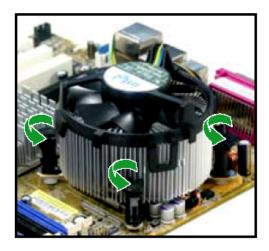
4. Pull up two fasteners at a time in a diagonal sequence to disengage the heatsink and fan assembly from the mainboard.
