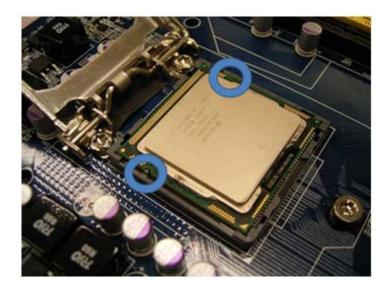
7. Close the "CPU Socket Cover" by lowering down the "CPU Socket Lever". Make sure the "CPU Socket Front Plates" are sliding underneath the "Shoulder Screw Cap".
