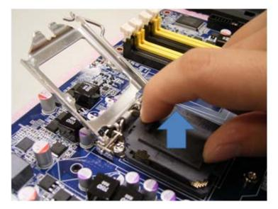
5. There are two notches on the CPU itself (one on each side), and there are two "Socket Alignment keys" on the CPU socket as well. Line up the two CPU notches with the "Socket Alignment Keys" on the socket, and insert the CPU into the CPU socket slowly.
