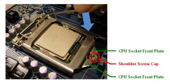
8. Secure the "CPU Socket Cover" by keep pressing down the "CPU Socket Lever" and move it toward and underneath the "Load Plate Tab".
