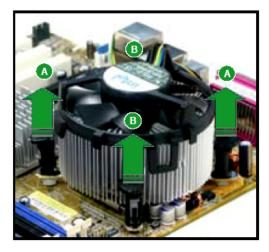
5. Rotate each fastener clockwise to ensure correct orientation when reinstalling.
