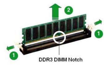
2. Remove the DIMM from the socket.
