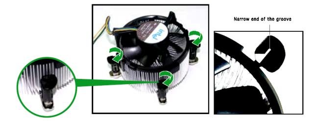
The narrow end of the groove should point outward after resetting. (The photo shows the groove shaded for emphasis.)
