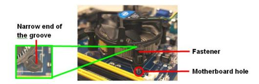
NOTE: Orient the heatsink and fan assembly so the CPU fan cable is close to the CPU fan connector).
