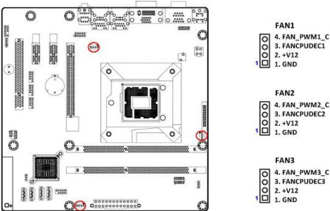
**Note:** FAN1 – CPU Fan; FAN2 – System Fan; FAN3 – Chassis Fan
