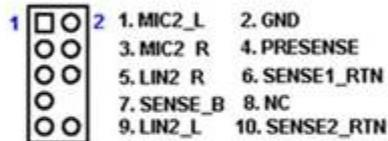
For motherboards with the optional HD Audio feature, we recommend that you connect a high-definition front panel audio module to this connector to avail of the motherboard's high-definition audio capability.
