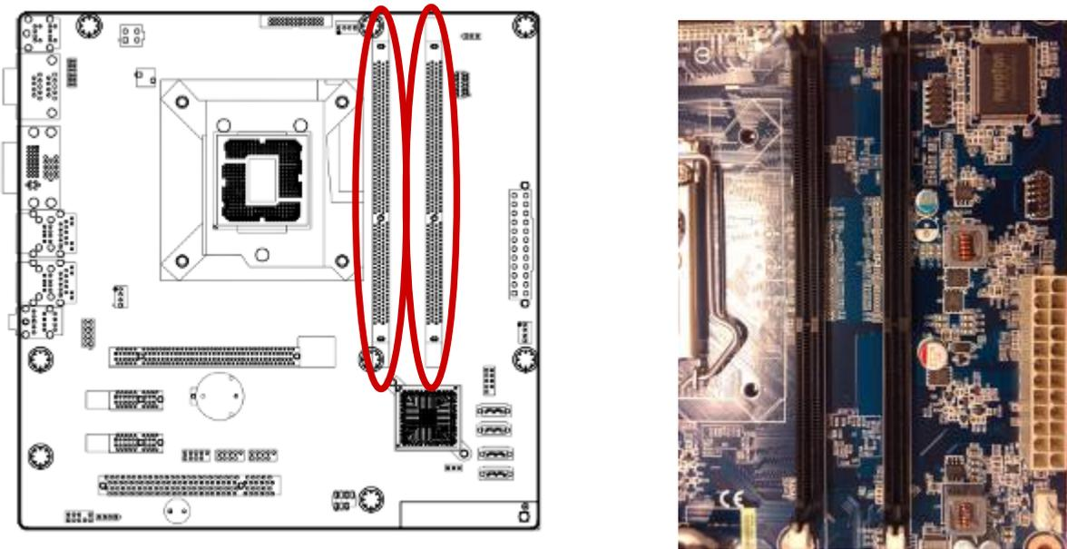
240-Pin DDR3 DIMM sockets
