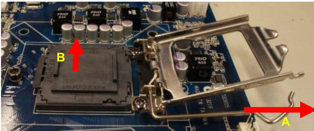
4. Position the CPU over the socket, making sure that the gold triangle is on the top-left corner of the socket then fit the socket alignment key into the CPU notch.
