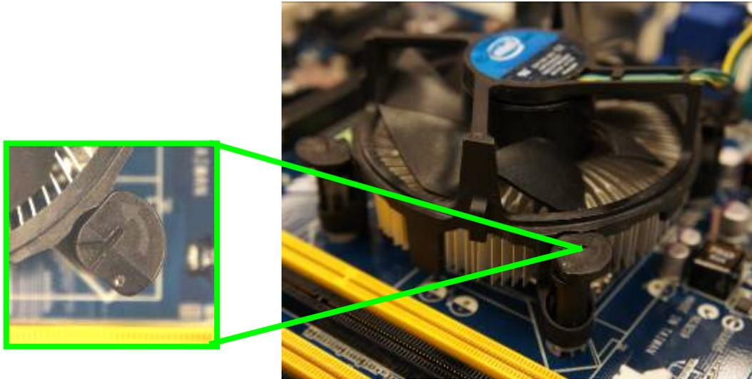
3. Pull up two fasteners at a time in a diagonal sequence to disengage the heatsink and fan assembly from the motherboard.
