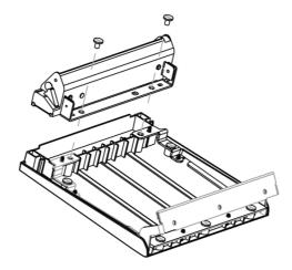
Step 4 Unscrew the two screws and the hex bolt to remove the printer assembly.
