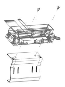
Step 6 Disconnect the two FPCs from the PCB.
