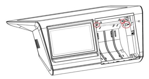
**Step 5** Unscrew two screws on the printer assembly to take down the printer module.
