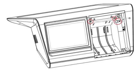
NOTE: Always install the hex bolt back before closing up the printer door.
