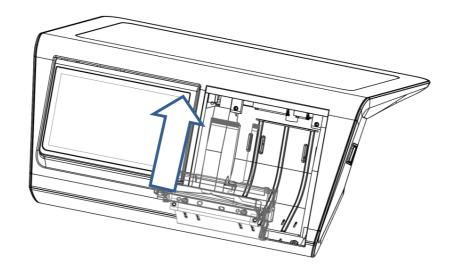
**Step 8** Use the screws to tie the printer module.
