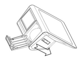
**Step 2** Unscrew the three screws that connects the printer doo to the device in order to take down the printer door.
