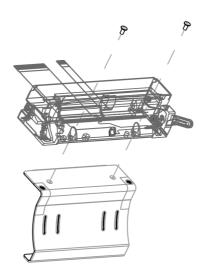
**Step 9** Install the printer assembly back into the device with the screws and insert the hex bolt back into place.
