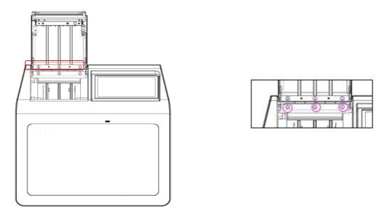
Step 3 Unscrew the two screws on the printer door to remove printer wheel.
