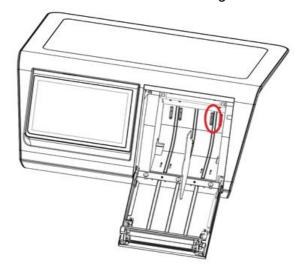
Load the paper roll to the left and close the printer door.
